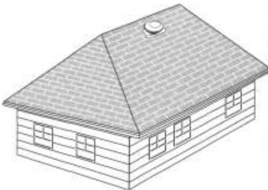
Figure 7-26: Power fans are used to move large volumes of air a good option for hard-to-vent hip roofs.
