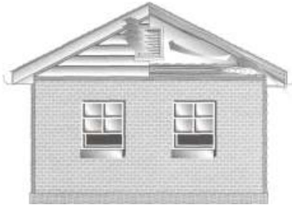
Figure 7-17: The gable-louver vent, an exhaust vent, allows unwanted air to flow out of the attic.
