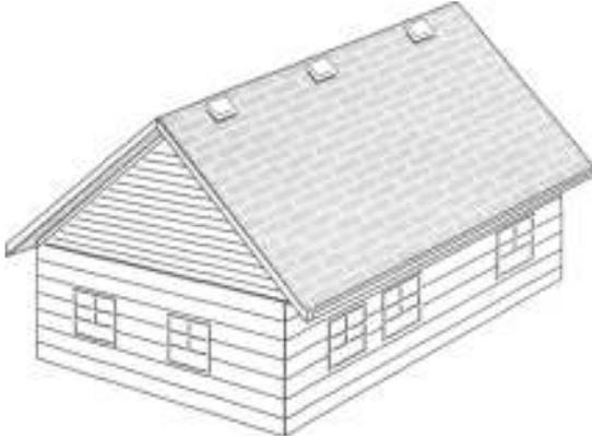
Figure 7-16: A roof vent is an exhaust vent located near the ridge.
