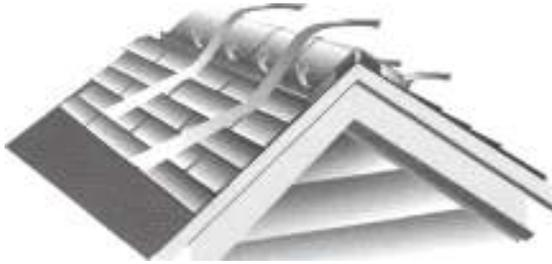
Figure 7-23: An externally baffled vent "pulls" air from the attic through both side of the vent.
