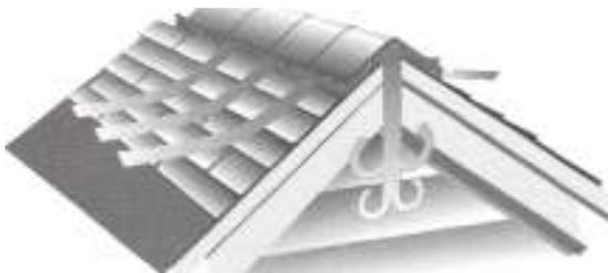
*Figure 7-22: A roll vent with an internal baffle, or without any baffle at all, does not "pull" air from the attic through both sides of the vent.*
