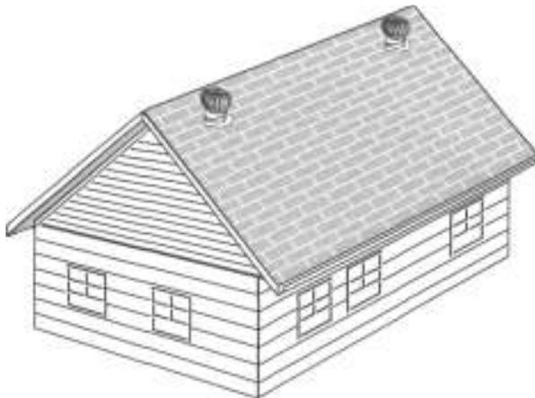
Figure 7-25: Wind turbines are located near the ridge and are used to exhaust air from the attic.
