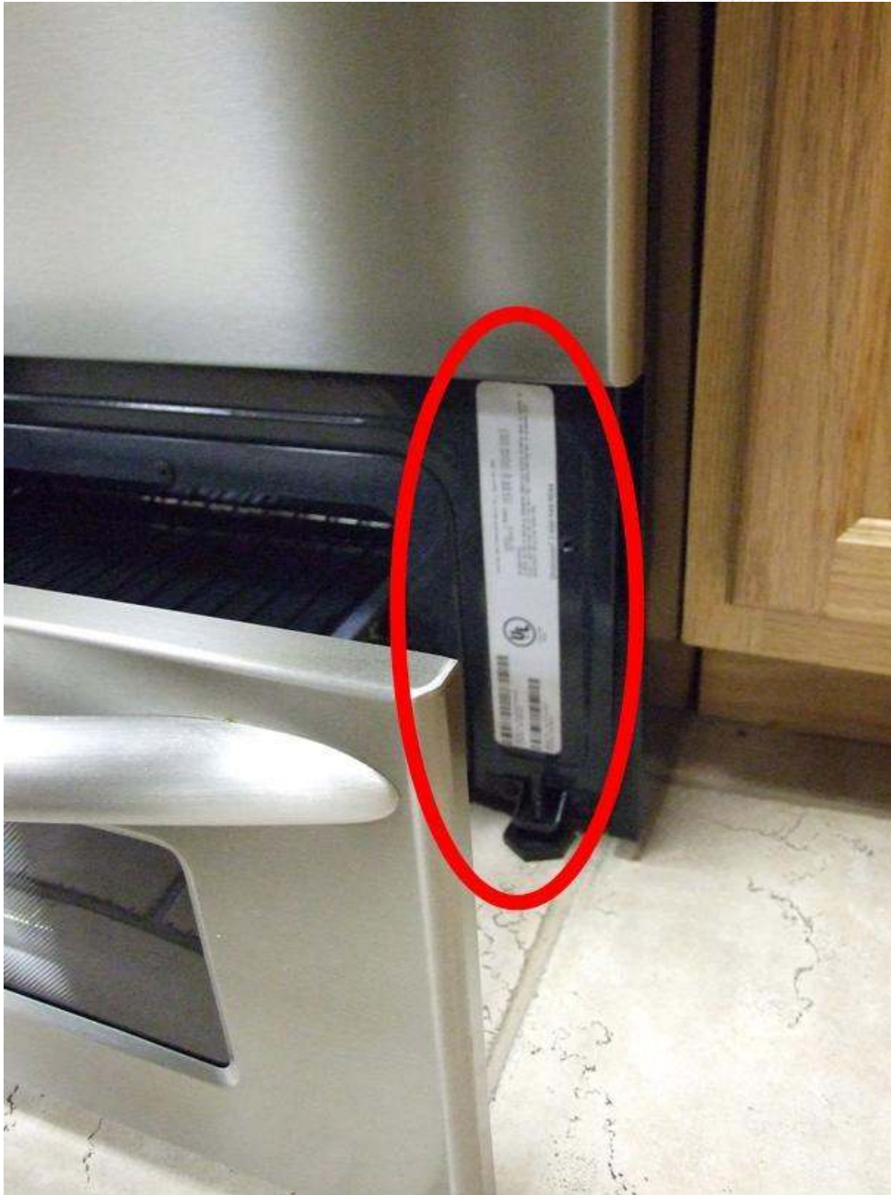
Serial plate is located by opening the range drawer at the bottom of the unit.
