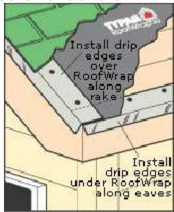
Installing drip edges:
